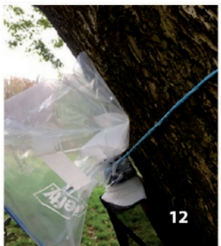
12. Cut along the edges of the zip-type bag just enough to slip it over the plastic top. Secure it with a zip-tie. 13. The finished trap secured to a tree.
