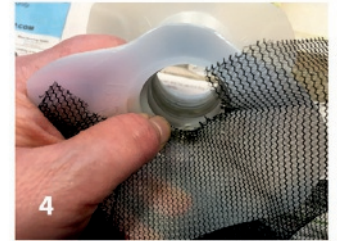
3. Fold screening and cut a small half circle out at the top. 4. Attach top of half circle of the screening to the inside of the milk jugs with a hot glue gun. Work slowly all the way around waiting for the glue to dry before attaching more.
